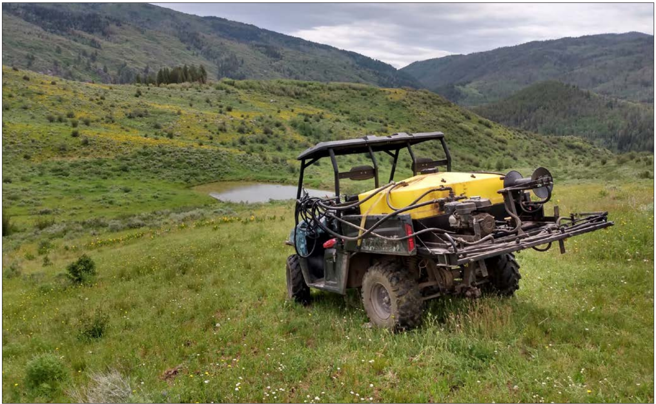
Figure 3.21. Utility Terrain Vehicle with herbicide spray tank and hose reel for targeted weed treatments in Route County, Colorado. (Photo: Todd Hagenbuch.)
